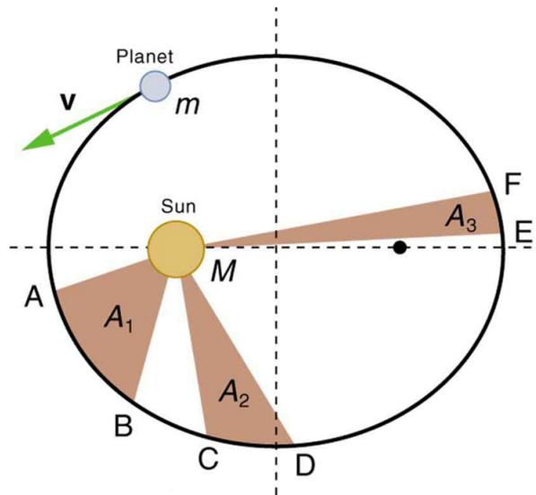
*The shaded regions have equal areas. It takes equal times for  $m$  to go from A to B, from C to D, and from E to F. The mass  $m$  moves fastest when it is closest to M. Kepler's second law was originally devised for planets orbiting the Sun, but it has broader validity.*
