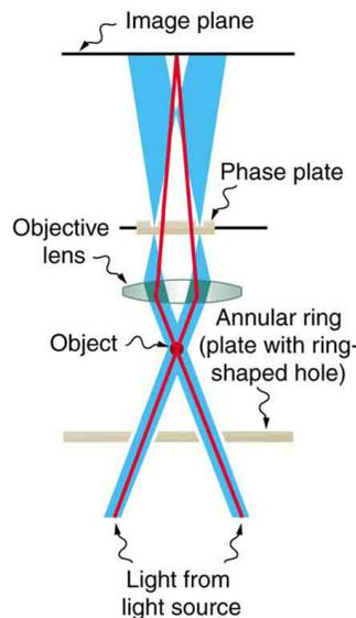
*Simplified construction of a phase-contrast microscope. Phase differences between light passing through the object and background are produced by passing the rays through different parts of a phase plate. The light rays are superimposed in the image plane, producing contrast due to their interference.*
