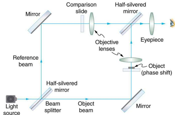
*An interference microscope utilizes interference between the reference and object beam to enhance contrast. The two beams are split by a half-silvered mirror; the object beam is sent through the object, and the reference beam is sent through otherwise identical optical elements. The beams are recombined by another half-silvered mirror, and the interference depends on the various phases emerging from different parts of the object, enhancing contrast.*
