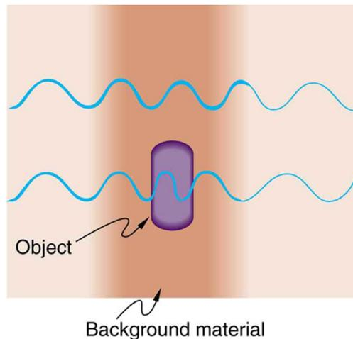
*Light rays passing through a sample under a microscope will emerge with different phases depending on their paths. The object shown has a greater index of refraction than the background, and so the wavelength decreases as the ray passes through it. Superimposing these rays produces interference that varies with path, enhancing contrast between the object and background.*
