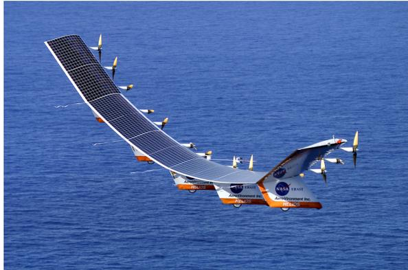
*Solar energy is converted into electrical energy by solar cells, which is used to run a motor in this solar-power aircraft. (credit: NASA)*
