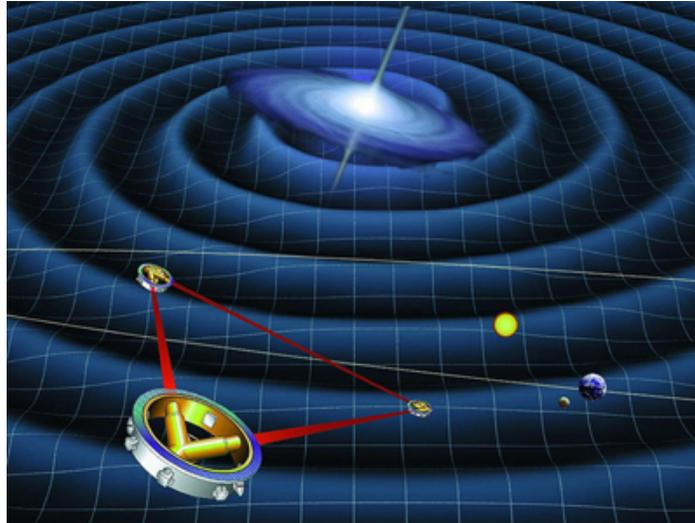
*Space-based future experiments for the measurement of gravitational waves. Shown here is a drawing of LISA’s orbit. Each satellite of LISA will consist of a laser source and a mass. The lasers will transmit a signal to measure the distance between each satellite’s test mass. The relative motion of these masses will provide information about passing gravitational waves.
