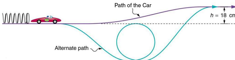
*A toy car is pushed by a compressed spring and coasts up a slope. Assuming negligible friction, the potential energy in the spring is first completely converted to kinetic energy, and then to a combination of kinetic and gravitational potential energy as the car rises. The details of the path*
