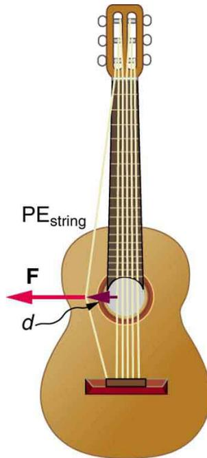
*Work is done to deform the guitar string, giving it potential energy. When released, the potential energy is converted to kinetic energy and back to potential as the string oscillates back and forth. A very small fraction is dissipated as sound energy, slowly removing energy from the string.*
