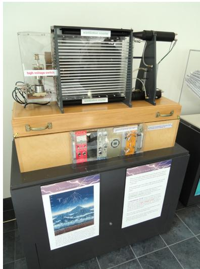
*A spark chamber is used to trace the paths of high-energy particles. Ionization created by the particles as they pass through the gas between the plates allows a spark to jump. The sparks are perpendicular to the plates, following electric field lines between them. The potential difference between adjacent plates is not high enough to cause sparks without the ionization produced by particles from accelerator experiments (or cosmic rays). (credit: Daderot, Wikimedia Commons)*
