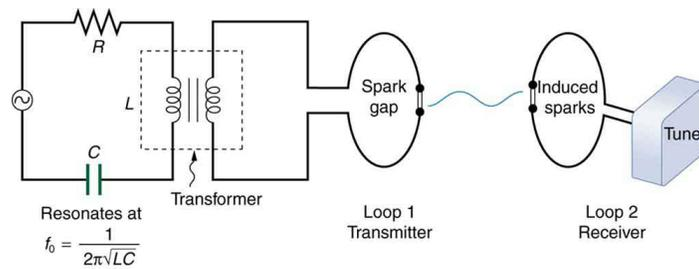
*The apparatus used by Hertz in 1887 to generate and detect electromagnetic waves. An RLC circuit connected to the first loop caused sparks across a gap in the wire loop and generated electromagnetic waves. Sparks across a gap in the second loop located across the laboratory gave evidence that the waves had been received.*
