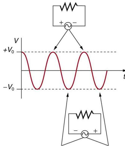
*The potential difference  $V$  between the terminals of an AC voltage source fluctuates as shown. The mathematical expression for  $V$  is given by  $V = V_0 \sin 2\pi ft$ .*
