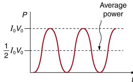
*AC power as a function of time. Since the voltage and current are in phase here, their product is non-negative and fluctuates between zero and  $I_0 V_0$ . Average power is  $(1/2)I_0 V_0$ .*
