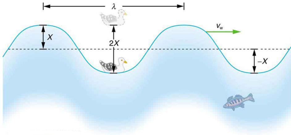
*An idealized ocean wave passes under a sea gull that bobs up and down in simple harmonic motion. The wave has a wavelength  $\lambda$ , which is the distance between adjacent identical parts of the wave. The up and down disturbance of the surface propagates parallel to the surface at a speed  $v_w$ .*
