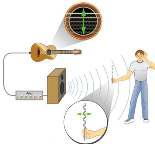
*The wave on a guitar string is transverse. The sound wave rattles a sheet of paper in a direction that shows the sound wave is longitudinal.*
