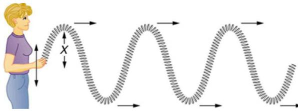
*In this example of a transverse wave, the wave propagates horizontally, and the disturbance in the cord is in the vertical direction.*
