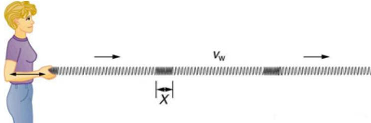
*In this example of a longitudinal wave, the wave propagates horizontally, and the disturbance in the cord is also in the horizontal direction.*
