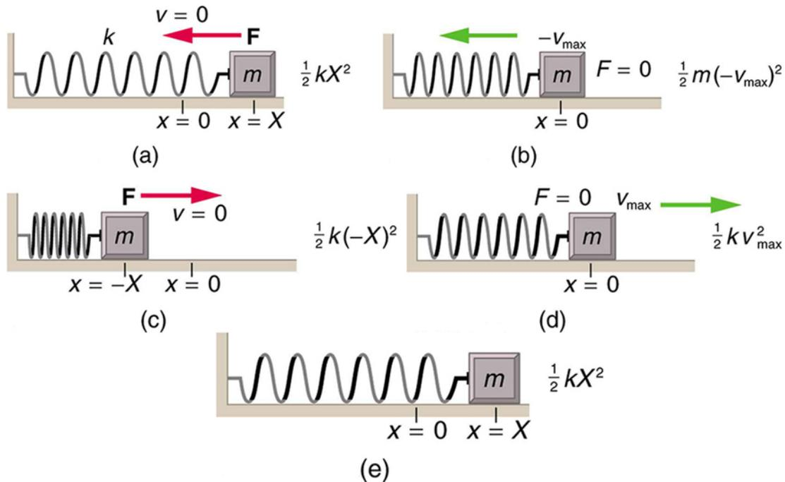
*The transformation of energy in simple harmonic motion is illustrated for an object attached to a spring on a frictionless surface.*
