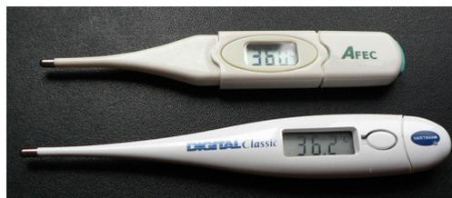
*These familiar thermometers are based on the automated measurement of a thermistor's temperature-dependent resistance. (credit: Biol, Wikimedia Commons)*
