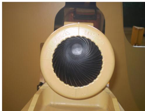
*The image shows a view down the barrel of a cannon, emphasizing its rifling. Rifling in the barrel of a canon causes the projectile to spin just as is the case for rifles (hence the name for the grooves in the barrel). (credit: Elsie esq., Flickr)*
