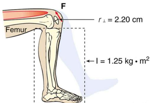
*The muscle in the upper leg gives the lower leg an angular acceleration and imparts rotational kinetic energy to it by exerting a torque about the knee.  $\tau$  is a vector that is perpendicular to  $r$ . This example examines the situation.*
