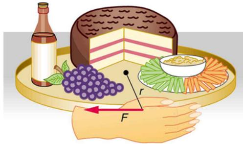
*A partygoer exerts a torque on a lazy Susan to make it rotate. The equation  $\text{net } \tau = \frac{\Delta L}{\Delta t}$  gives the relationship between torque and the angular momentum produced.*
