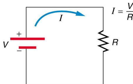
*A simple electric circuit in which a closed path for current to flow is supplied by conductors (usually metal wires) connecting a load to the terminals of a battery, represented by the red parallel lines. The zigzag symbol represents the single resistor and includes any resistance in the connections to the voltage source.*
