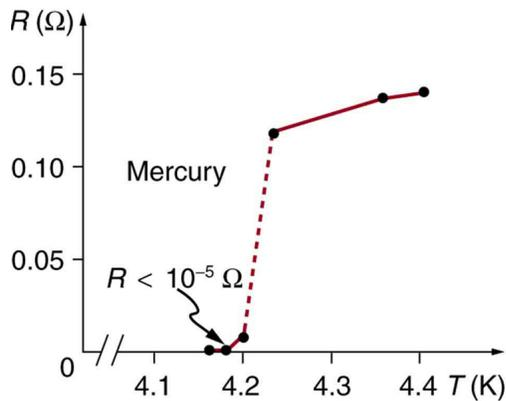
*A graph of resistivity versus temperature for a superconductor shows a sharp transition to zero at the critical temperature  $T_c$ . High temperature superconductors have verifiable  $T_c$  s greater than 125 K, well above the easily achieved 77-K temperature of liquid nitrogen.*
