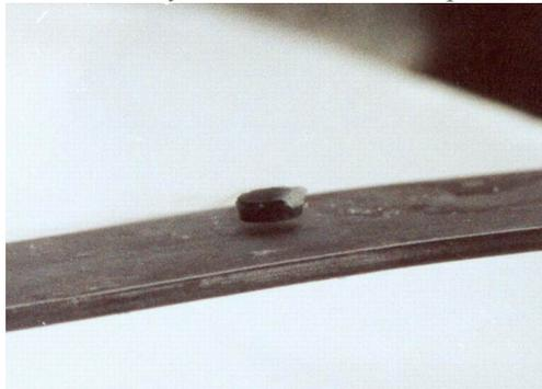
*One characteristic of a superconductor is that it excludes magnetic flux and, thus, repels other magnets. The small magnet levitated above a high-temperature superconductor, which is cooled by liquid nitrogen, gives evidence that the material is superconducting. When the material warms and becomes conducting, magnetic flux can penetrate it, and the magnet will rest upon it. (credit: Saperaud)*
