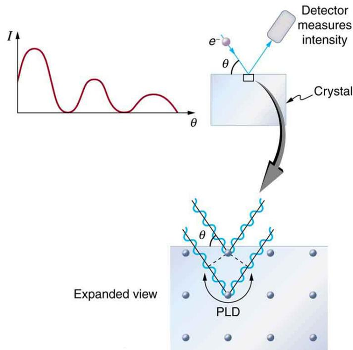
*The diffraction pattern at top left is produced by scattering electrons from a crystal and is graphed as a function of incident angle relative to the regular array of atoms in a crystal, as shown at bottom. Electrons scattering from the second layer of atoms travel farther than those scattered from the top layer. If the path length difference (PLD) is an integral wavelength, there is constructive interference.*
