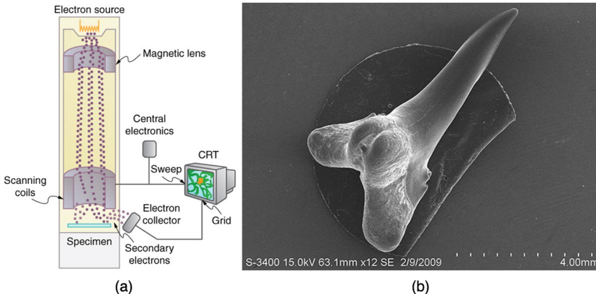
*Schematic of a scanning electron microscope (SEM) (a) used to observe small details, such as those seen in this image of a tooth of a Himipristis, a type of shark (b). (credit: Dallas Krentzel, Flickr)*
