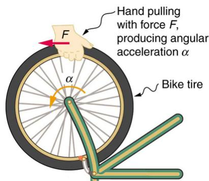
*Force is required to spin the bike wheel. The greater the force, the greater the angular acceleration produced. The more massive the wheel, the smaller the angular acceleration. If you push on a spoke closer to the axle, the angular acceleration will be smaller.*
