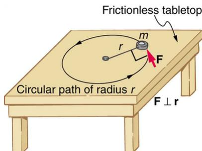
*An object is supported by a horizontal frictionless table and is attached to a pivot point by a cord that supplies centripetal force. A force  $F$  is applied to the object perpendicular to the radius  $r$ , causing it to accelerate about the pivot point. The force is kept perpendicular to  $r$ .*
