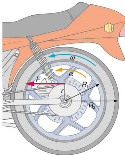
*A motorcycle wheel has a moment of inertia approximately that of an annular ring.*
