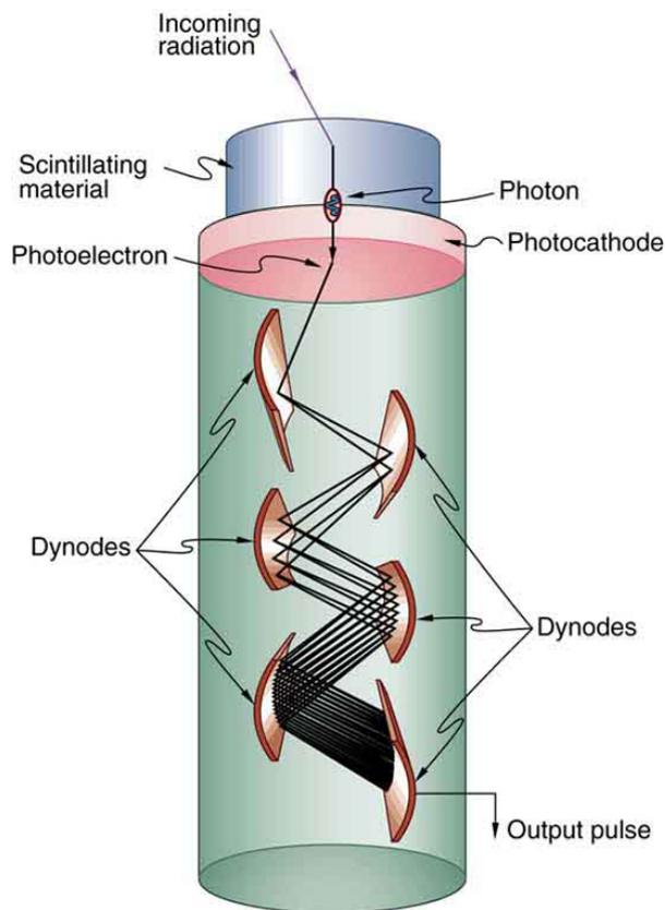
*Photomultipliers use the photoelectric effect on the photocathode to convert the light output of a scintillator into an electrical signal. Each successive dynode has a more-positive potential than the last and attracts the ejected electrons, giving them more energy. The number of electrons is thus multiplied at each dynode, resulting in an easily detected output current.*
