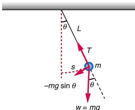
*A simple pendulum has a small-diameter bob and a string that has a very small mass but is strong enough not to stretch appreciably. The linear displacement from equilibrium is  $s$ , the length of the arc. Also shown are the forces on the bob, which result in a net force of  $-mg \sin \theta$  toward the equilibrium position—that is, a restoring force.*
