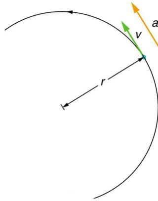
*In circular motion, linear acceleration  $a$ , occurs as the magnitude of the velocity changes:  $a$  is tangent to the motion. In the context of circular motion, linear acceleration is also called tangential acceleration  $a_t$ .*
