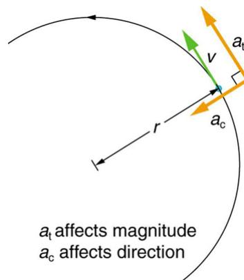
*Centripetal acceleration  $a_c$  occurs as the direction of velocity changes; it is perpendicular to the circular motion. Centripetal and tangential acceleration are thus perpendicular to each other.*
