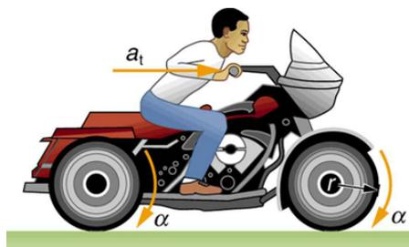
*The linear acceleration of a motorcycle is accompanied by an angular acceleration of its wheels.*
