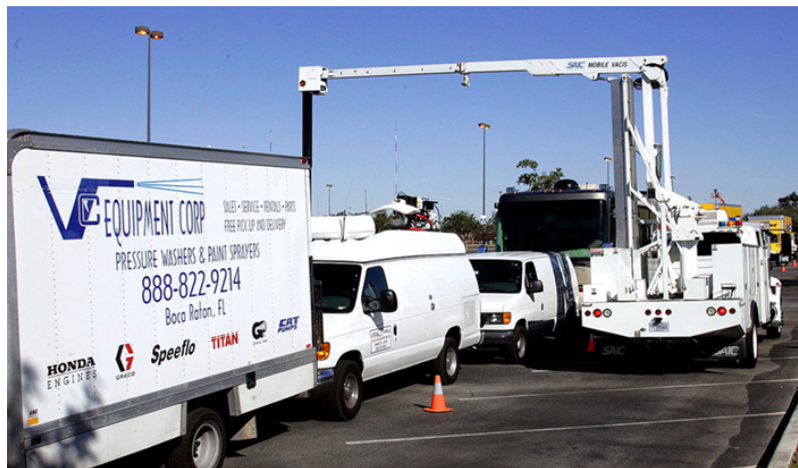
Customs officers inspect vehicles using neutron irradiation. Cars and trucks pass through portable x-ray machines that reveal their contents. (credit: Gerald L. Nino, CBP, U.S. Dept. of Homeland Security)
