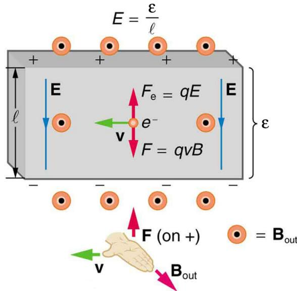
*The Hall emf  $\epsilon$  produces an electric force that balances the magnetic force on the moving charges. The magnetic force produces charge separation, which builds up until it is balanced by the electric force, an equilibrium that is quickly reached.*
