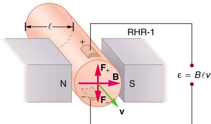
*The Hall effect can be used to measure fluid flow in any fluid having free charges, such as blood. The Hall emf  $\epsilon$  is measured across the tube perpendicular to the applied magnetic field and is proportional to the average velocity  $v$ .*
