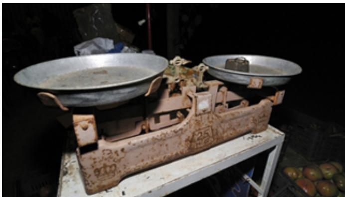
*A double-pan mechanical balance is used to compare different masses. Usually an object with unknown mass is placed in one pan and objects of known mass are placed in the other pan. When the bar that connects the two pans is horizontal, then the masses in both pans are equal. The “known masses” are typically metal cylinders of standard mass such as 1 gram, 10 grams, and 100 grams. (credit: Serge Melki)*
