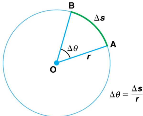
*The radius of a circle is rotated through an angle  $\Delta\theta$ . The arc length  $\Delta s$  is described on the circumference.*
