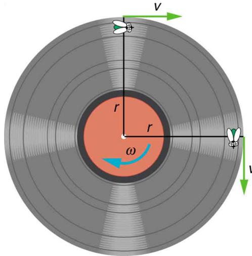
*As an object moves in a circle, here a fly on the edge of an old-fashioned vinyl record, its instantaneous velocity is always tangent to the circle. The direction of the angular velocity is clockwise in this case.*
