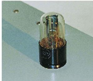
*The photoelectric effect can be observed by allowing light to fall on the metal plate in this evacuated tube. Electrons ejected by the light are collected on the collector wire and measured as a current. A retarding voltage between the collector wire and plate can then be adjusted so as to determine the energy of the ejected electrons. For example, if it is sufficiently negative, no electrons will reach the wire. (credit: P.P. Urone)*
